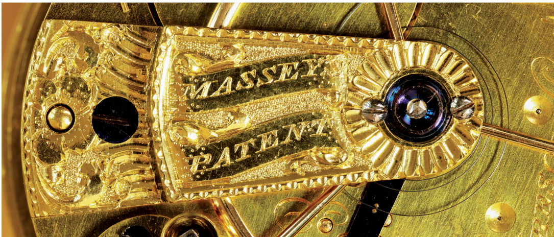
Balance cock, engraved 'Massey Patent', on a previously unrecorded seconds beating watch by Edward Massey, Prescott, hallmarked Chester 1821. Photograph Charles Frodsham & Co.
