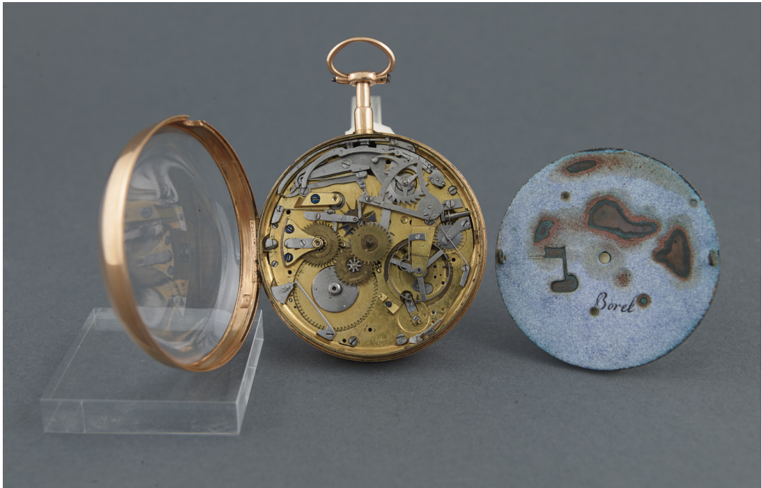
Perpetuelle watch (self winding) with repetition of hours and quarters. Abraham-Louis Breguet, Paris, 1797. Gold. Ø 52 mm. Movement signed 'N.34 Inventé par Breguet à Paris', dial signed 'Breguet et Fils'. Mark on the case: 34. Inv. 6004. Donation from the Luigi Delle Piane collection, 2017.
