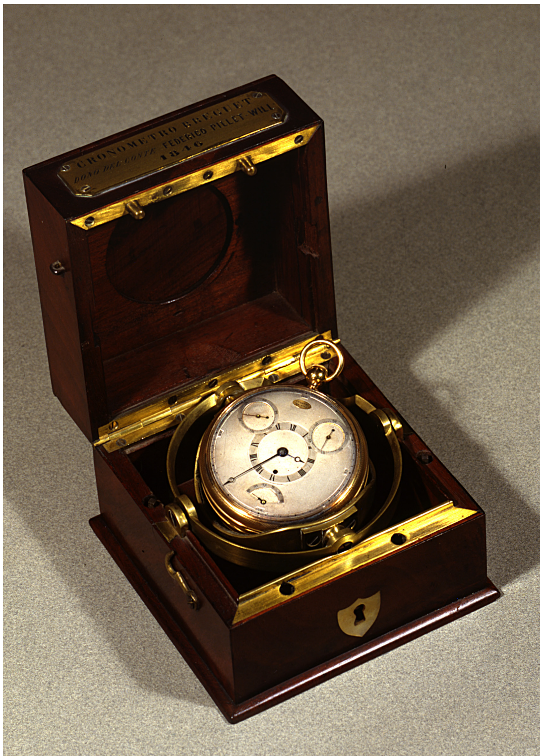
Pocket chronometer Ø 64 mm, mounted in gimbals, by Abraham-Louis Breguet, Paris, 1806-1815. Inv. 3565-3566. Inscribed 'Breguet N. 2180'. Donated by the Academy of Science at Turin in 1975.
