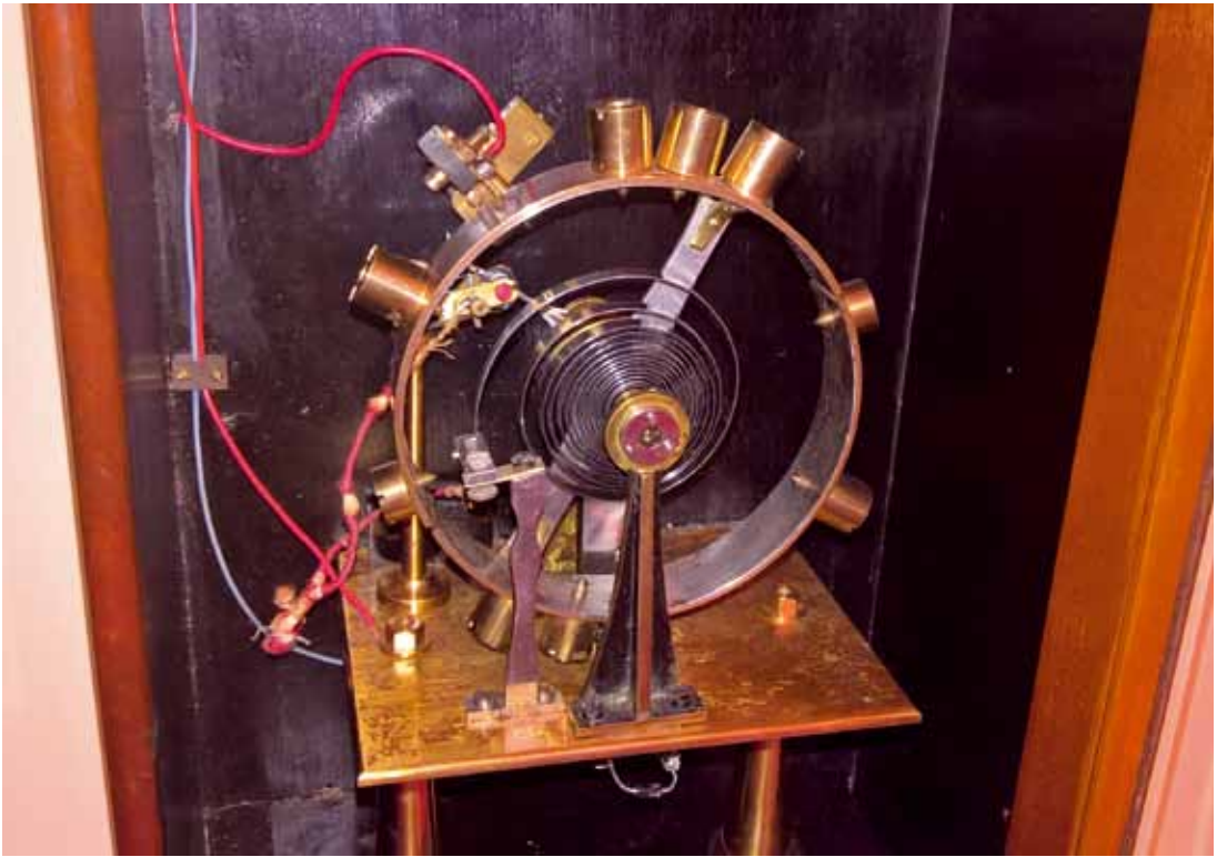
Fig. 10. The large balance wheel. Note the redundant contact block on the backboard.
