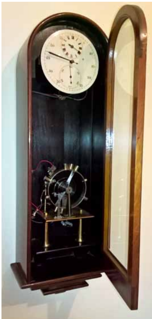
Fig. 8. The electric balance wheel clock or, in his own words, the 'large balance precision timekeeper' from Stanley Wise's own collection.
