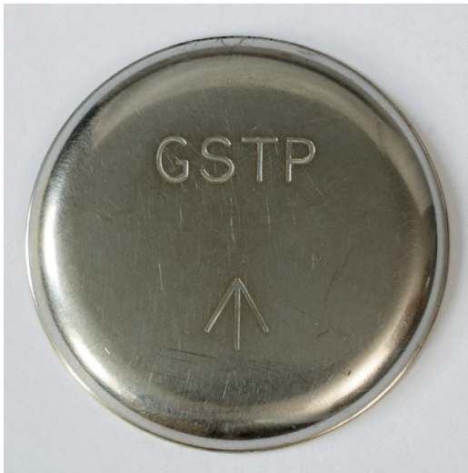
Figs 3 and 4. Back and movement of the pocket watch shown in Fig. 2. It was made for the Army from 1942 in accordance with the General Service Trade Pattern specification.
