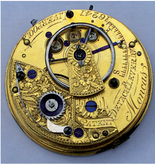
Fig. 12. Late full-plate movement with Massey type III detached lever escapement. Signed: Moncas, Liverpool, 16241. Manufactured post 1832. Photo © Michael W. Paice.
