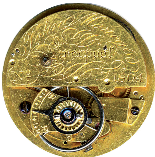
Fig. 4. Very early half-plate movement with Massey type I detached lever escapement. Signed: John Moncas, Liverpool, No. 1804. Manufactured in 1820. Photo courtesy of and © Alan Treherne.
