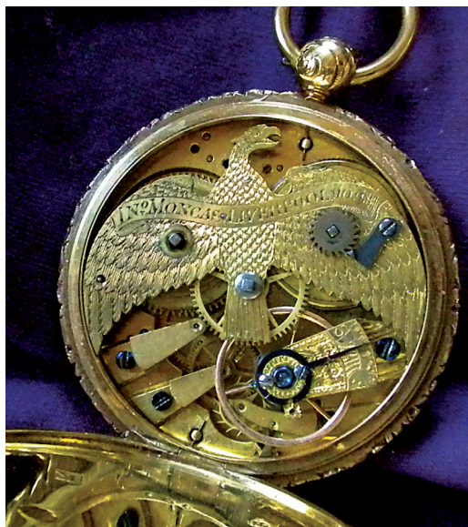
Fig. 6. Right-angled single table half-plate lever movement, with three arm balance. Signed: John Moncas, Liverpool, 9098. Photo courtesy of and © Doug Cowan.
