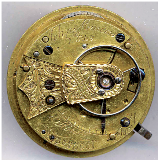
Fig. 2. Early full-plate lever watch movement. Signed: John Moncas, Liverpool, 549. Manufactured in 1815 whilst still at the Hanover Street address. Photo courtesy of and © Alan Treherne.
