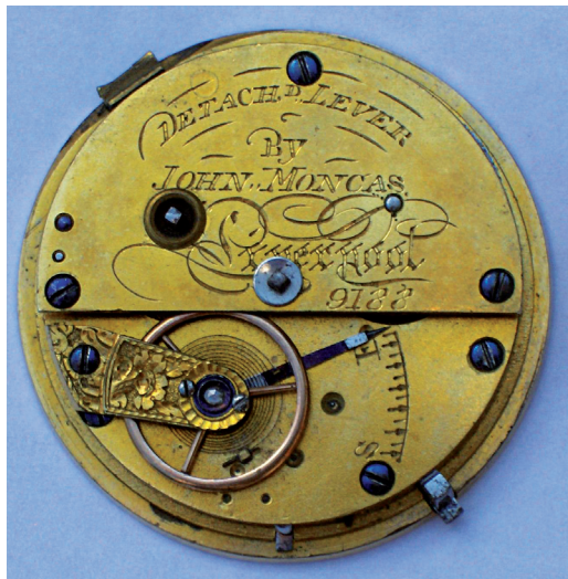
Fig. 3. Split-plate movement with Massey type II detached lever escapement. Signed John Moncas, Liverpool, 9188. Manufactured 1828/29. Photo © Michael W. Paice.
