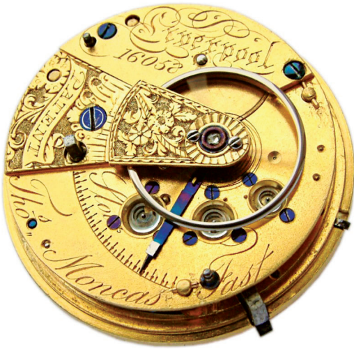
Fig. 10. Late full-plate movement with Massey type III detached lever escapement. Signed: Thos. Moncas, Liverpool, 16058. Manufactured circa 1832. Photo courtesy of and © Peter Marsh.
