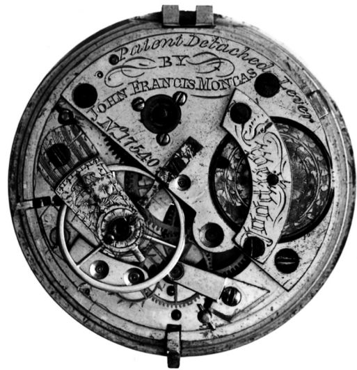
Fig. 13. Half-plate lever movement, with three arm balance. Harrison's maintaining power, engraved cap to barrel and escapement to separate cocks. Signed: John Francis Moncas, Liverpool, No. 17540. Manufactured circa 1837. Photo © Trustees of the British Museum.
