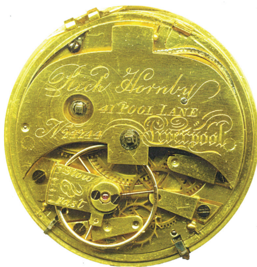
Fig. 7. Richard Hornby movement showing unfinished phoenix/eagle styled half-plate. Photo courtesy of and © Alan Treherne.
