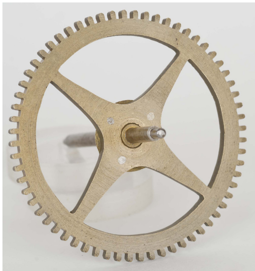
Fig. 10. A detail view of the striking 2nd wheel showing the pin-rivets that secure the wheel to the rear of the lantern pinion shroud.
