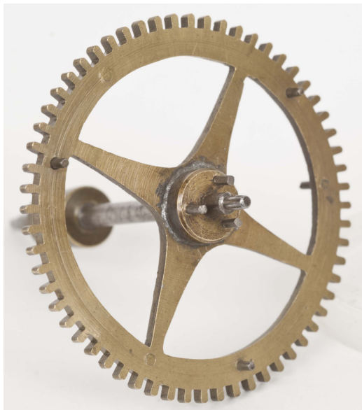
Fig. 14. A detail view of the rear side of the striking 3rd wheel showing the three sets of three pins.
