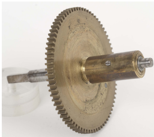
Fig. 8. A detail view of the rear face of the striking great wheel with the mainspring removed. Note how two brass tubes have been positioned over the steel arbor, one over the other, to increase the arbor's diameter (with the spring hooking piece secured through all the thicknesses of material). Exactly the same constructional technique was used on the going great wheel.
