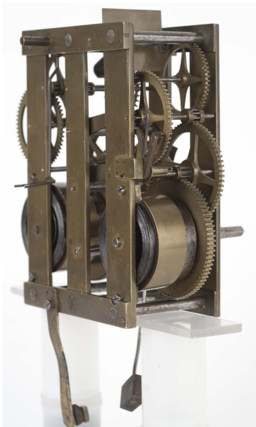
Fig. 1. A \frac{3}{4} left rear movement view showing the rear strip plate construction and the striking train wheels. Note the two screws that secure the striking mainspring's cast brass containing ring in place, both being on the rear right vertical strip plate.
