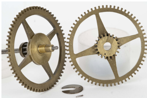
Fig. 13. A detailed view of the going 2nd wheel with intermediate wheel assembly completely dismantled from the arbor.
