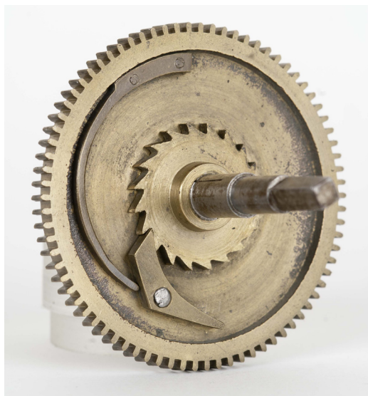
Fig. 7. A detailed view of the front face of the striking great wheel showing the use of typical English click work. (The click work on the going great wheel is exactly the same but reversed.)
