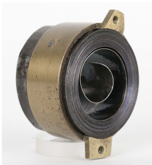
Fig. 9. A detailed view of the striking mainspring cast brass retaining ring removed from the movement but with the mainspring still installed within the retaining ring. (The cast brass retaining ring for the going mainspring is exactly the same as this one but with minor lug-shaping differences; the direction of the spring is also reversed.)
