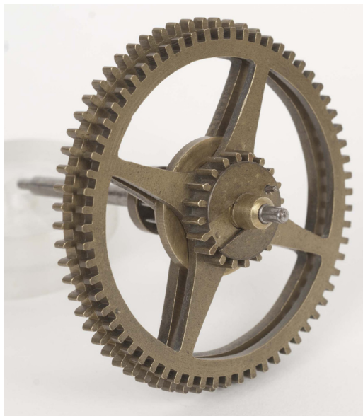
Fig. 12. A detail view of the going 2nd wheel with the intermediate wheel assembly secured to the arbor. Note the witness marks on both intermediate wheel and pinion at an 8 o'clock position and how the tips of the intermediate wheel have been topped; these topped teeth provide clearance with the 3rd wheel's lantern pinion shroud when this wheel is assembled in the movement (see Figures 2 & 4).
